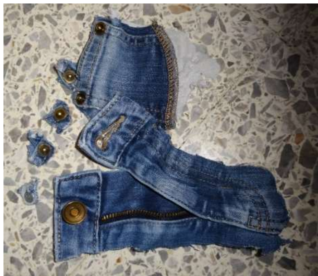
Figure 7 Removal of metal parts
