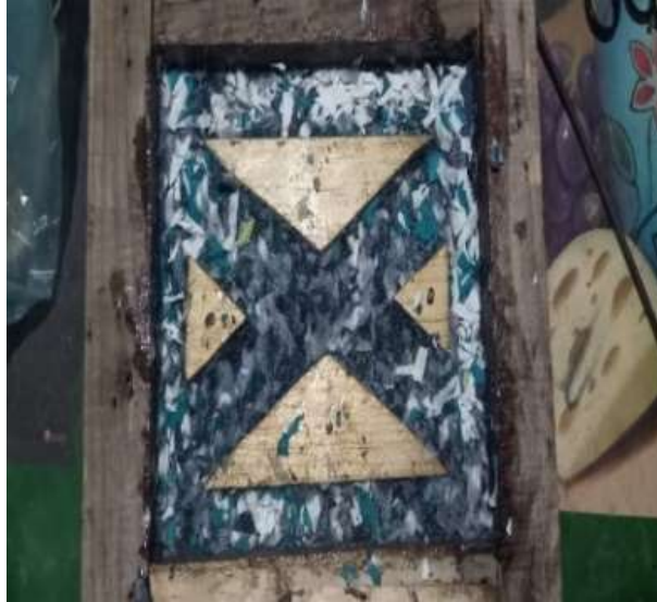
Figure 12 Pressure is applied to the entire mixture
